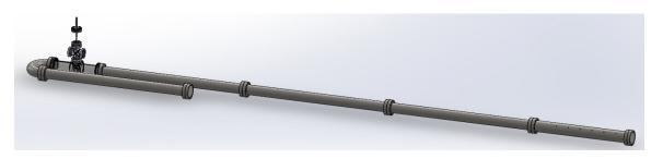
Figure 2.16: Brown Shock Tube, single-pulse constant-area driver solid model
